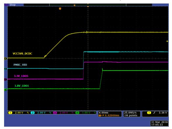
Figure 8. Power-On Sequence for the TPS65911x Voltage Rails
