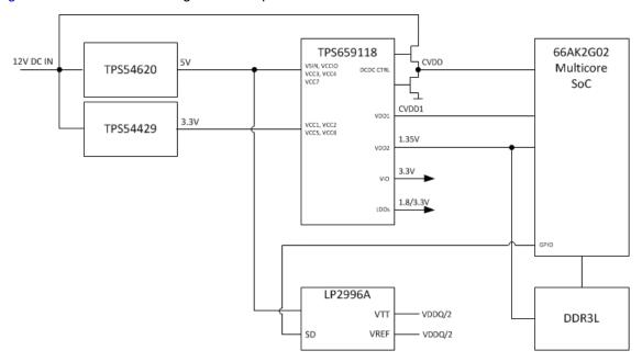
Figure 1. K2G General Purpose EVM Power Solution Block Diagram
