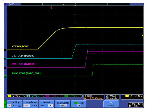
Figure 6. Power-On Sequence for the TPS65911x
