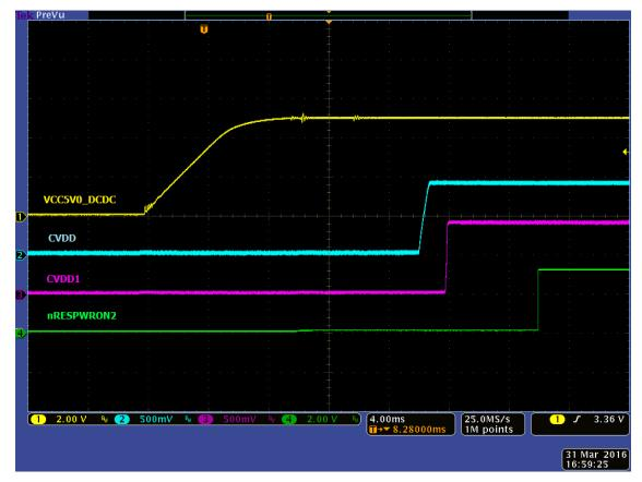
Figure 7. Power-On Sequence for the TPS65911x With nRESPWRON2
