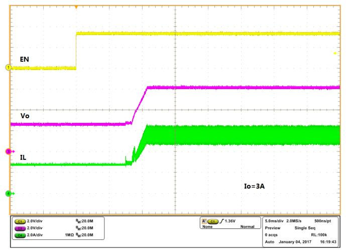
Figure 4. Start-up Waveforms at  $I_o = 3 A (V_o = 9 V)$
