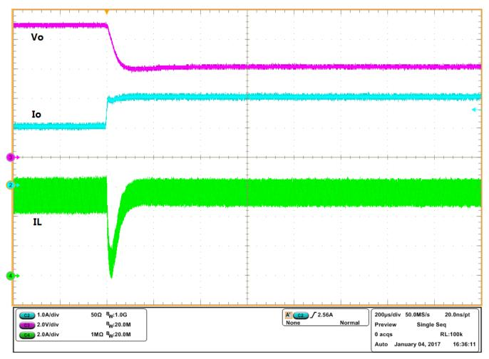
Figure 5. Output Current Limit Waveforms at V<sub>o</sub> = 9 V (Io = 2 A to 3 A)
