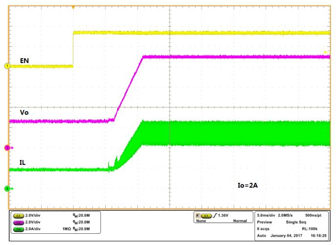
Figure 3. Start-up Waveforms at  $I_0 = 2 A (V_0 = 9 V)$
