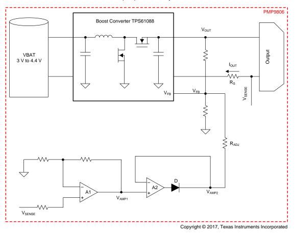
Figure 1. PMP9806 Block Diagram
