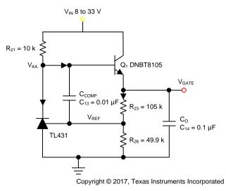
Figure 18. Gate Voltage Supply
