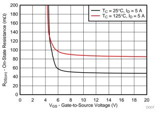
Figure 14. MOSFET On-State Resistance
