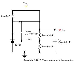
Figure 19. Peripheral Supply
