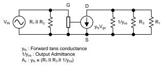
Figure 24. AC Equivalent Circuit
