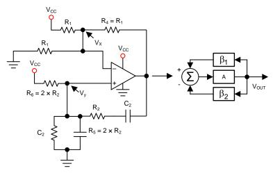
Figure 21. Sine Wave Oscillator for Op Amp
