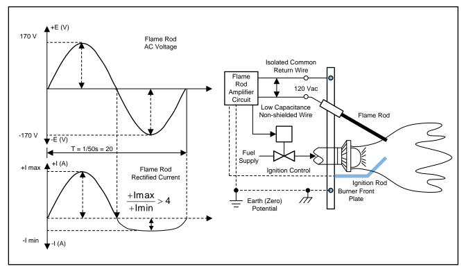
Figure 2. Flame Sensing Using Flame Rod
