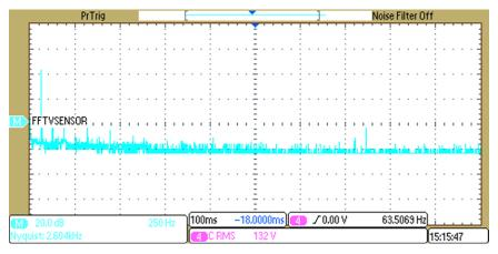
Figure 37. FFT Plot Sensor Output
