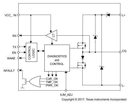
Figure 2. Block Diagram of TIOL111
