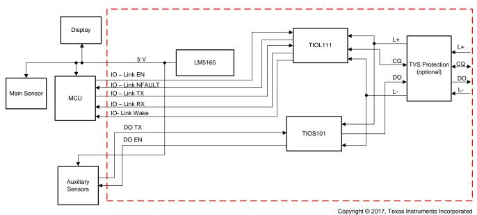
Figure 1. TIDA-01478 Block Diagram
