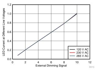
Figure 24. External Dimming Signal versus LED Current at Different Line Voltages
