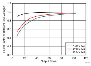
Figure 22. Output Power versus Power Factor at Different Line Voltages
