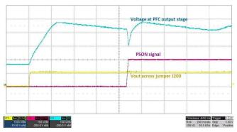
Figure 33. Start-up at 120-V AC With No Load at Output
