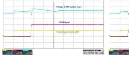
Figure 37. Start-up at 265-V AC With No Load at Output
