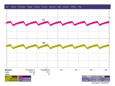
Figure 32. Output Voltage and Current Ripple With 196-W LED Load at 265-V AC
