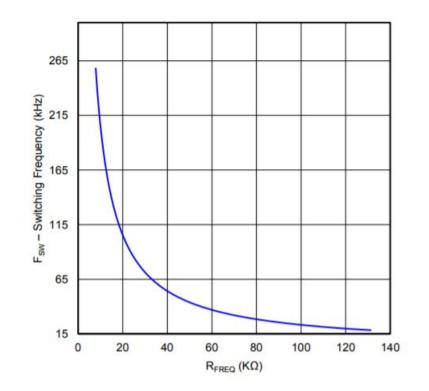
Figure 10. Frequency versus R<sub>FREQ</sub>
