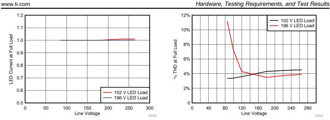
Figure 14. Line Voltage versus LED Current at Full Load
