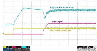
Figure 34. Start-up at 120-V AC With 196-W LED Load at Output
