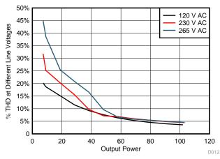
Figure 23. Output Power versus THD at Different Line Voltages
