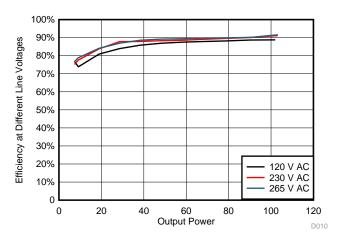
Figure 21. Output Power versus Efficiency at Different Line Voltages
