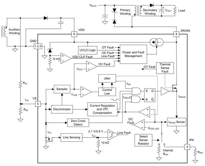
Figure 6. UCC28910 Functional Block Diagram
