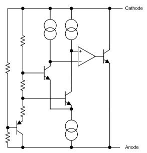
Figure 9. LM4040 Functional Block Diagram
