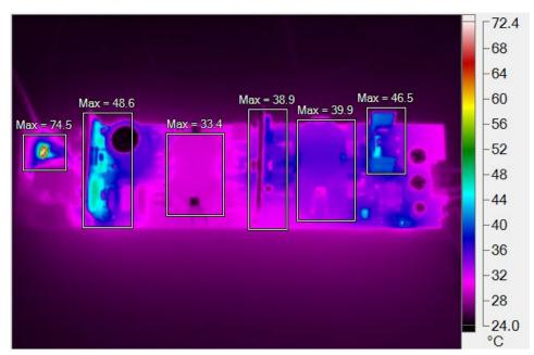
Figure 42. Thermal Image of Top View of TIDA-01464 PCB With 196-W Load at 230-V Input AC Voltage
