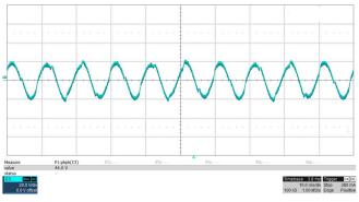
Figure 29. PFC Output Ripple at 120-V AC With 196-W LED Load
