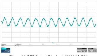
Figure 28. PFC Output Ripple at 120-V AC With 196-W LED Load
