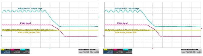
Figure 39. Turnoff at 120-V AC With 196-W LED Load at Output
