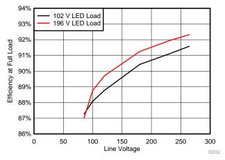
Figure 13. Line Voltage versus Efficiency at Full Load
