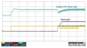
Figure 36. Start-up at 230-V AC With 196-W LED Load at Output
