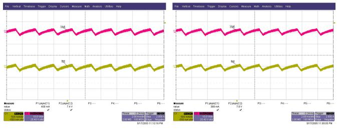
Figure 30. Output Voltage and Current Ripple With 196-W LED Load at 120-V AC
