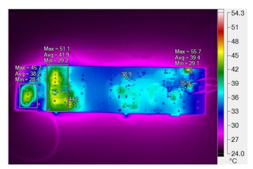
Figure 43. Thermal Image of Bottom View of TIDA-01464 PCB With 196-W Load at 230-V Input AC Voltage
