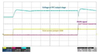
Figure 35. Start-up at 230-V AC With No Load at Output
