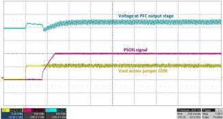
Figure 38. Start-up at 265-V AC With 196-W LED Load at Output
