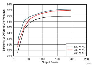
Figure 17. Output Power versus Efficiency at Different Line Voltages
