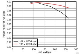
Figure 16. Line Voltage versus Power Factor at Full Load
