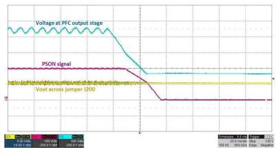
Figure 41. Turnoff at 265-V AC With 196-W LED Load at Output
