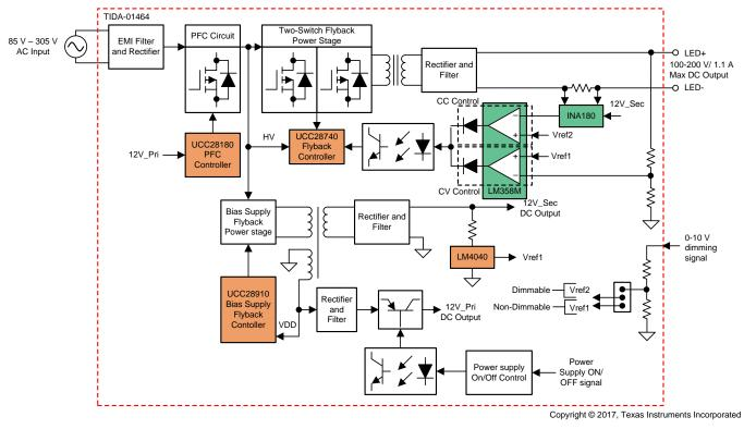
Figure 3. TIDA-01464 Block Diagram
