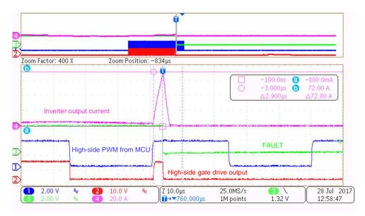
Figure 47. Zoomed View of Overcurrent Latch Protection With Motor Stall by V<sub>DS</sub> Monitoring
