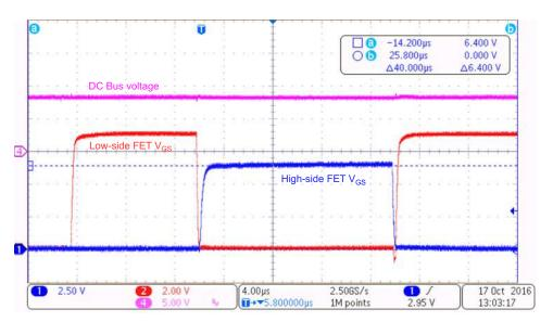
Figure 19. High- and Low-Side Gate Drive Voltage at 8-V DC
