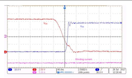
Figure 23. Turnoff: Low-Side  $V_{\rm gs}$  and  $V_{\rm Ds}$  at 18-A Winding Current
