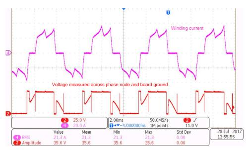
Figure 26. Load Test Results at 36-V DC Input, 17.4-A<sub>RMS</sub> Winding Current, 100% Duty Cycle
