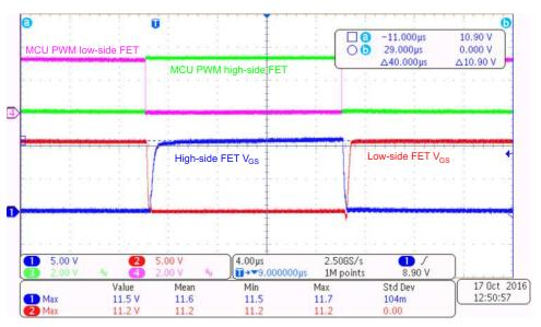
Figure 18. Low- and High-Side Gate Drive Voltage at 36-V DC
