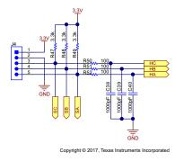
Figure 8. Schematic of Hall Sensor Connector
