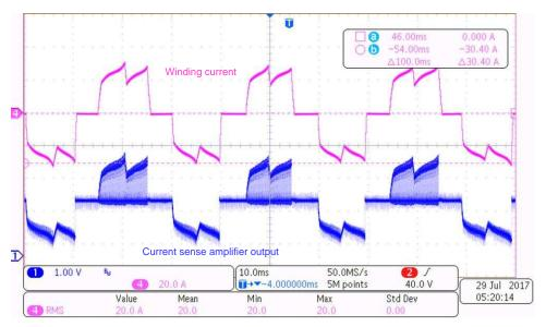
Figure 38. DRV8323 Current Sense Amplifier Output at 52% Duty Cycle
