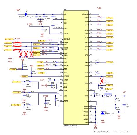
Figure 5. Schematic of DRV8323 Gate Driver
