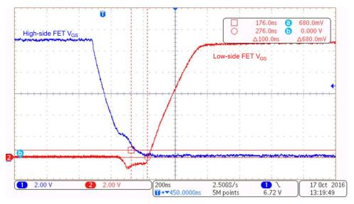
Figure 20. Dead Time at Rising Edge of Low-Side V<sub>GS</sub>
