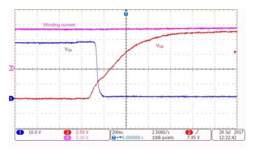
Figure 24. Turnon: High-Side  $V_{\rm GS}$  and  $V_{\rm DS}$  at 14-A Winding Current
