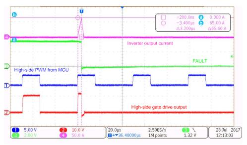
Figure 48. Overcurrent Latch Protection With Inverter Output Shorted
