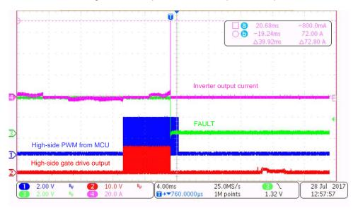
Figure 46. Overcurrent Latch Protection With Motor Stall by V<sub>DS</sub> Monitoring
