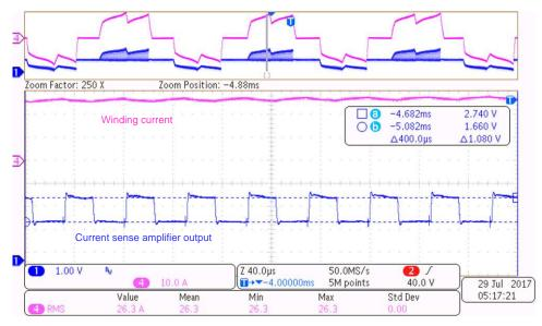
Figure 39. PWM Cycle View of DRV8323 Current Sense Amplifier Output at 52% Duty Cycle
