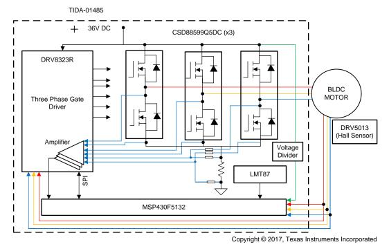
Figure 1. Block Diagram of TIDA-01485
