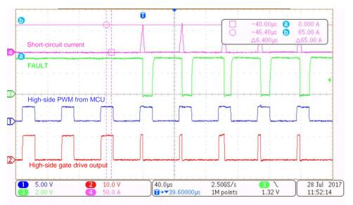
Figure 43. Cycle-by-Cycle Overcurrent Protection With Inverter Output Shorted
