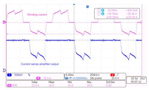
Figure 37. DRV8323 Current Sense Amplifier Output at 100% Duty Cycle
