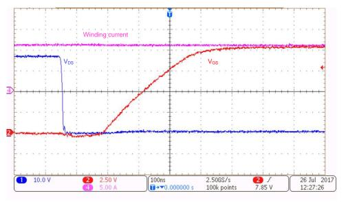
Figure 22. Turnon: Low-Side  $V_{\rm GS}$  and  $V_{\rm DS}$  at 12-A Winding Current
