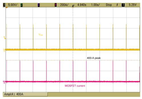
Figure 55. Multiple-Pulse Peak Current Testing With 400 A for 10 ms With 1% Duty Cycle (990 ms off)
