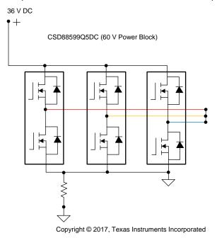
Figure 42. Test Setup to Simulate Inverter Short Circuit
