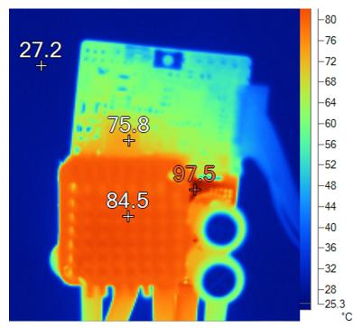
Figure 31. Thermal Image at 36-V DC Input, 25.3-A<sub>RMS</sub> Winding Current, 95% Duty Cycle
