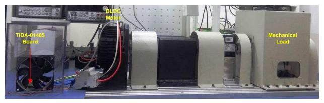
Figure 15. Board and Motor Test Setup
