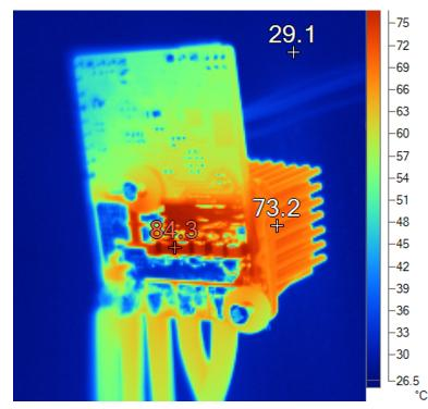
Figure 57. Thermal Image of Board at 850 W, Showing Effective Top-Side Cooling
