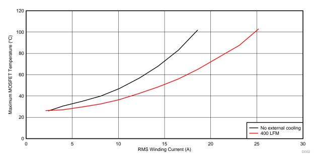
Figure 33. Load Test Results at 36-V DC Input, 95% Duty Cycle Without Heat Sink at Different Airflow
