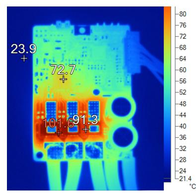
Figure 29. Thermal Image at 36-V DC Input, 18.6- $A_{RMS}$  Winding Current, 95% Duty Cycle
