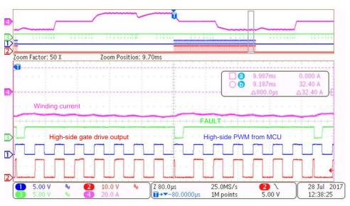
Figure 41. Cycle-by-Cycle Overcurrent Limit Showing PWM Shutoff
