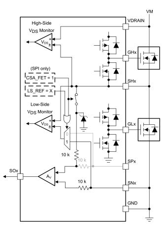
Figure 6. DRV8323 Current Shunt Amplifier Simplified Block Diagram
