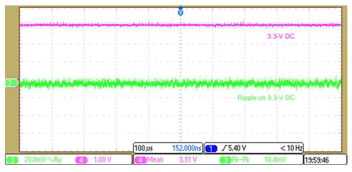
Figure 16. Output Voltage of 3.3 V From Step-Down Converter and 3.3-V Voltage Ripple
