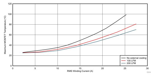
Figure 35. Load Test Results at 36-V DC Input, 95% Duty Cycle With Heat Sink at Different Airflow
