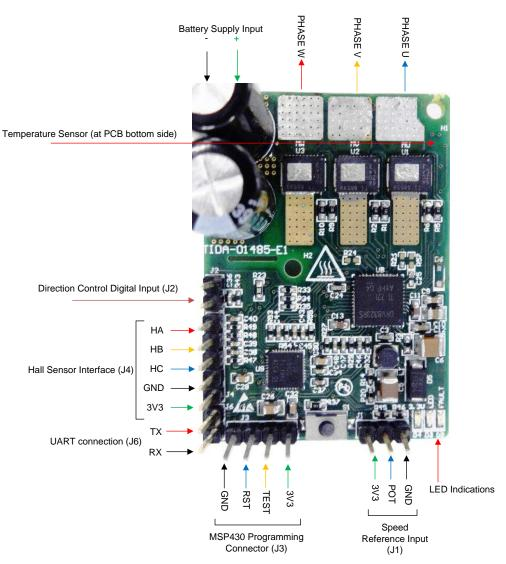
Figure 13. TIDA-01485 PCB Connectors
