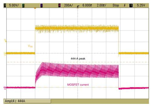
Figure 54. Single-Pulse Peak Current Testing With 400 A for 10 ms
