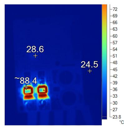
Figure 52. Thermal Image of Board After 400 ms With 100-A Peak Current in Motor Winding
