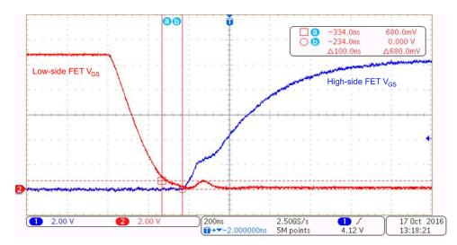
Figure 21. Dead Time at Trailing Edge of Low-Side V<sub>gs</sub>
