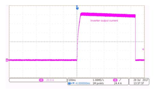
Figure 51. Peak Current of 100-A Peak Current in Motor Winding During Motor Stall
