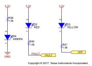
Figure 12. Schematic of LED Indications
