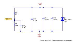
Figure 2. Schematic of Battery Power Input Section
