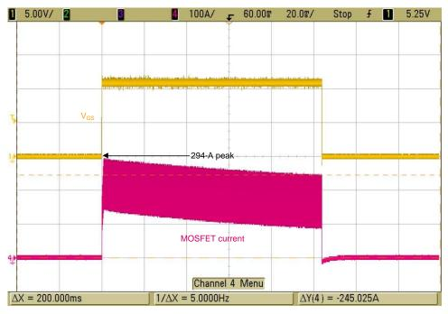
Figure 53. Single-Pulse Peak Current Testing With 200 A for 100 ms
