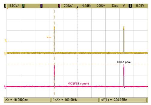
Figure 56. Multiple-Pulse Peak Current Testing With 400 A for 10 ms With 1% Duty Cycle (Zoomed)
