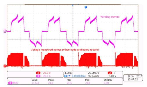
Figure 28. Load Test Results at 36-V DC Input, 18.6-A<sub>RMS</sub> Winding Current, 95% Duty Cycle
