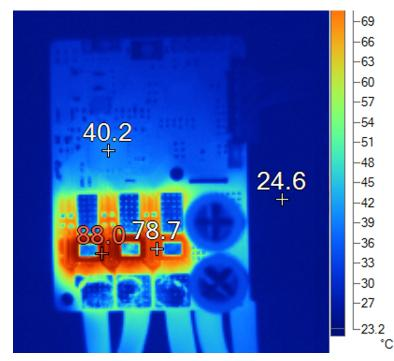
Figure 27. Thermal Image at 36-V DC Input, 17.4-A<sub>RMS</sub> Winding Current, 100% Duty Cycle
