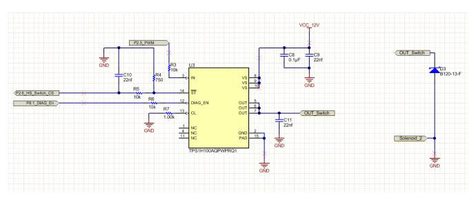
Figure 5. High-Side Switch Schematics
