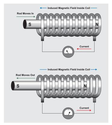
Figure 2. Working Solenoid
