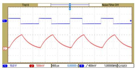
Figure 21. 50% Duty cycle—PWM Input versus Current Shunt Output, Ch 1: PWM Input, Ch 2: INA240-Q1 Output
