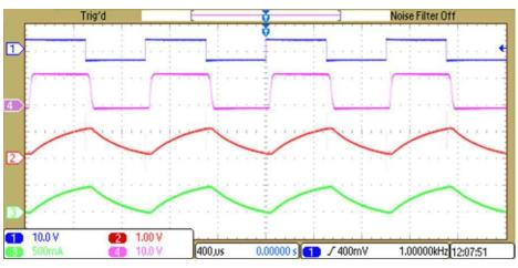
Figure 13. 50% Duty Cycle—Ch 1: Input PWM, Ch 2: INA240-Q1 Output, Ch 3: Current Probe Output, Ch 4: 12-V Pulsating
