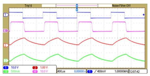
Figure 12. 40% Duty Cycle—Ch 1: Input PWM, Ch 2: INA240-Q1 Output, Ch 3: Current Probe Output, Ch 4: 12-V Pulsating
