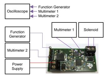
Figure 7. TIDA-01506 Hardware Setup
