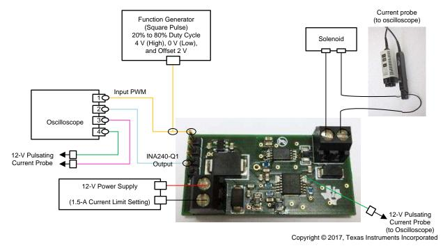
Figure 8. PWM Operation of Solenoid
