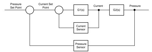
Figure 3. Closed-Loop Solenoid Control
