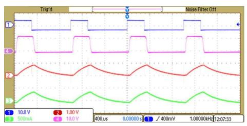
Figure 11. 30% Duty Cycle—Ch 1: Input PWM, Ch 2: INA240-Q1 Output, Ch 3: Current Probe Output, Ch 4: 12-V Pulsating
