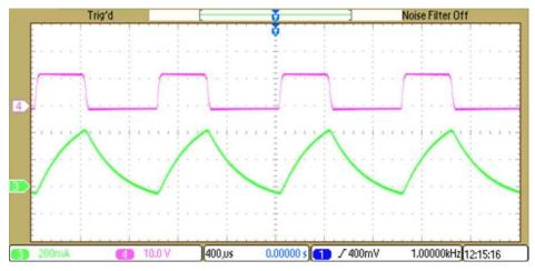
Figure 17. 40% Duty Cycle—Ch 4: Pulsating DC, Ch 3: Current Through Solenoid
