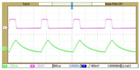
Figure 16. 20% Duty Cycle—Ch 4: Pulsating DC, Ch 3: Current Through Solenoid
