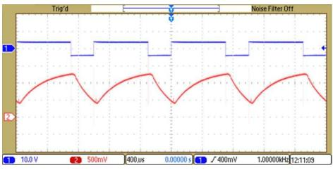
Figure 23. 80% Duty cycle—PWM Input versus Current Shunt Output, Ch 1: PWM Input, Ch 2: INA240-Q1 Output
