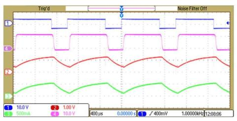
Figure 15. 70% Duty Cycle—Ch 1: Input PWM, Ch 2: INA240-Q1 Output, Ch 3: Current Probe Output, Ch 4: 12-V Pulsating
