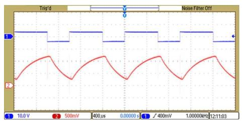
Figure 22. 60% Duty cycle—PWM Input versus Current Shunt Output, Ch 1: PWM Input, Ch 2: INA240-Q1 Output
