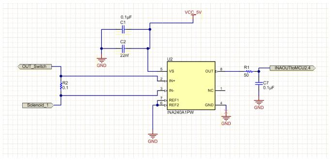
**Figure 4. Current Shunt Monitor Schematics**
