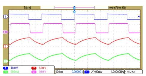
Figure 14. 60% Duty Cycle—Ch 1: Input PWM, Ch 2: INA240-Q1 Output, Ch 3: Current Probe Output, Ch 4: 12-V Pulsating
