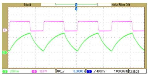
Figure 18. 60% Duty Cycle—Ch 4: Pulsating DC, Ch 3: Current Through Solenoid
