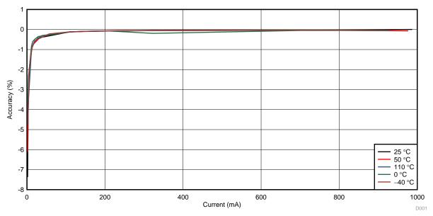
Figure 25. FS Accuracy at Different Temperatures
