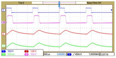
Figure 10. 20% Duty Cycle—Ch 1: Input PWM, Ch 2: INA240-Q1 Output, Ch 3: Current Probe Output, Ch 4: 12-V Pulsating
