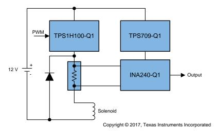
Figure 1. TIDA-01506 Block Diagram
