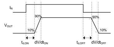
Figure 6. TPS1H100-Q1 Switching Characteristics Diagram
