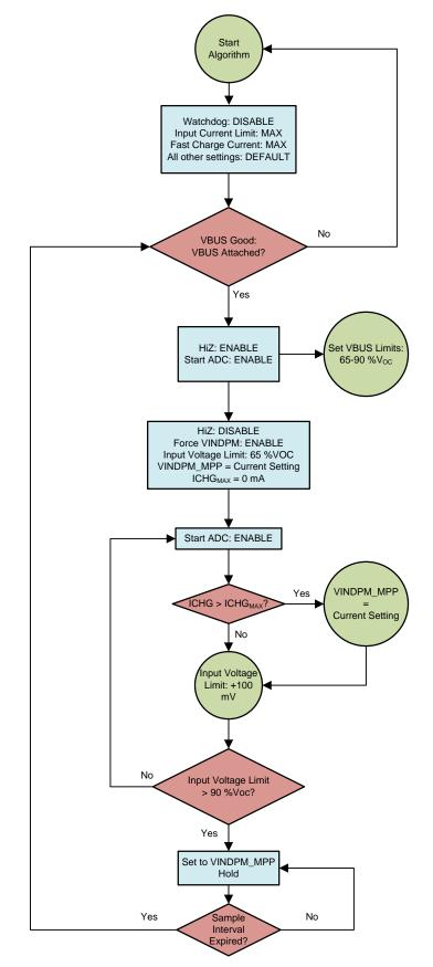
Figure 2. MPPT Algorithm Flow Diagram
