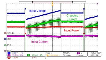
Figure 12. MPPT Range—Low Input Current:  $I_{sc}$  = 0.15 A, V<sub>oc</sub> = 10 V
