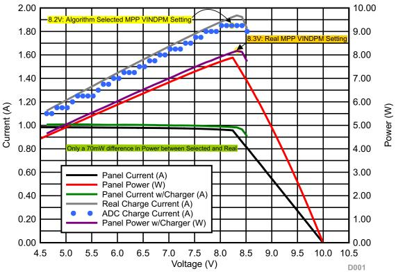
(10V V<sub>OC</sub>, 1A I<sub>SC</sub>, 3.8V V<sub>BAT</sub>)
