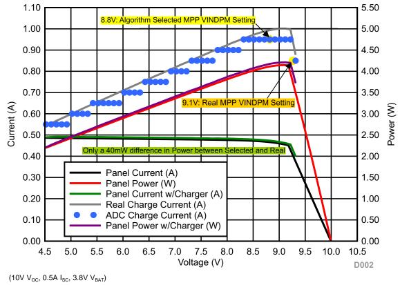
Figure 5. Moderate Irradiance Simulation—MPPT Performance
