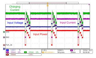
Figure 11. MPPT Range—Low Input Voltage:  $V_{oc}$  = 4.5 V,  $I_{sc}$  = 0.5 A Showing Input Power
