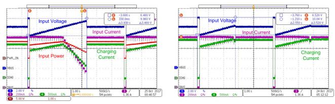
Figure 8. MPPT Without Tracking Time Optimization
