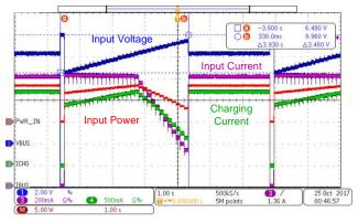
Figure 6. Tracking Loop Range—Lower Limit
