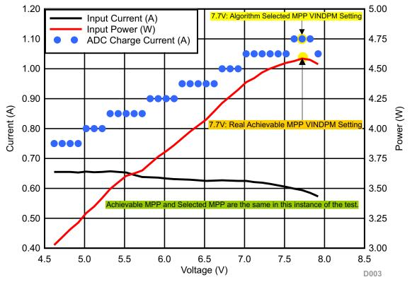
(9.5V<sub>OC</sub>, 0.65A I<sub>SC</sub>, 3.1V<sub>BAT</sub>, 6Ah Battery)
