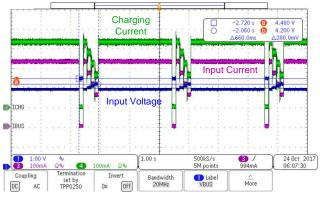
Figure 10. MPPT Range—Low Input Voltage:  $V_{oc}$  = 4.5 V,  $I_{sc}$  = 0.5 A
