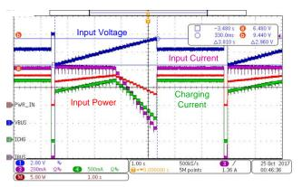
Figure 7. Tracking Loop Range—Upper Limit
