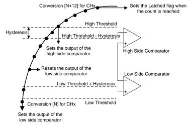
Figure 10. Thresholds and Hysteresis for Digital Window Comparator
