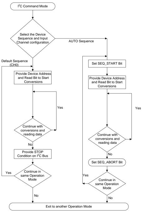
Figure 16. Device Operation in I<sup>2</sup>C Command mode
