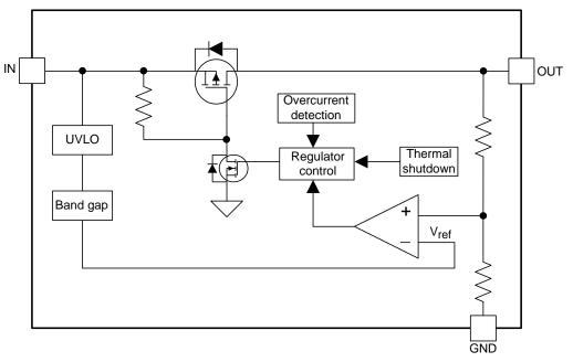
Figure 5. TPS7B69xx-Q1 Functional Block Diagram
