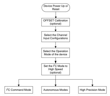
Figure 15. Configuring Device Into Different Modes
