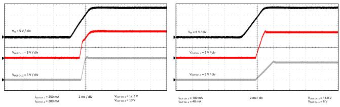
Figure 18. Ch.1 and Ch.2 Start-Up Waveform
