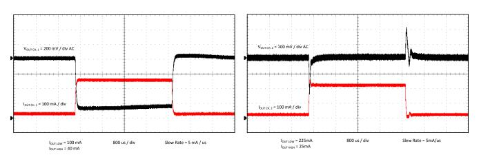
Figure 20. Ch.1 Load Transient Performance
