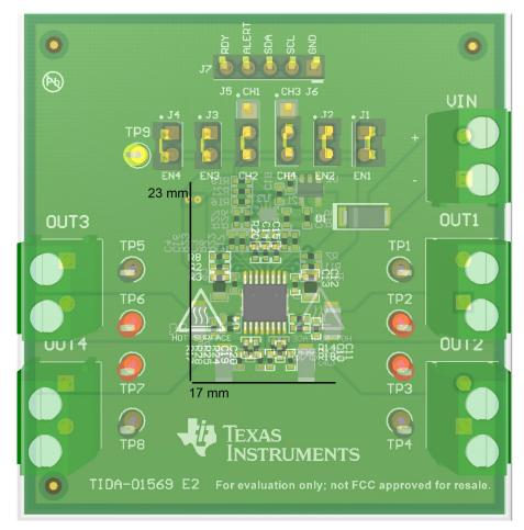
Figure 7. TIDA-01569 System Solution Size
