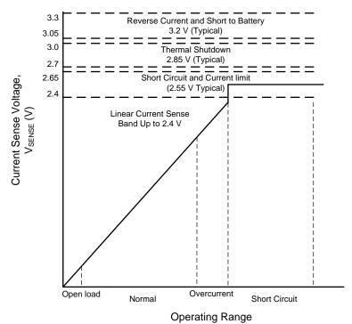
Figure 3. Functionality of Current-Sense Output
