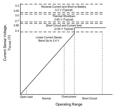
Figure 8. Analog Current Sense Output
