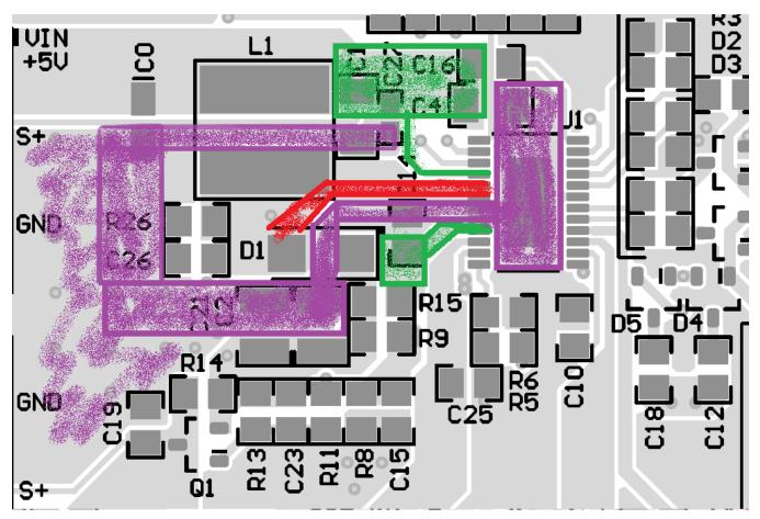
Figure 4. Layout of Correct Routing
