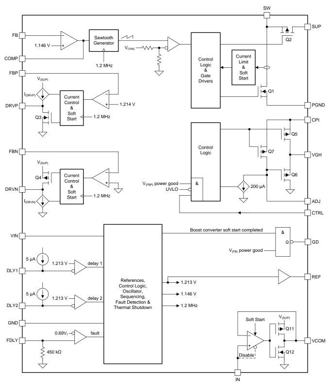
Figure 2. Block Diagram of TPS65150
