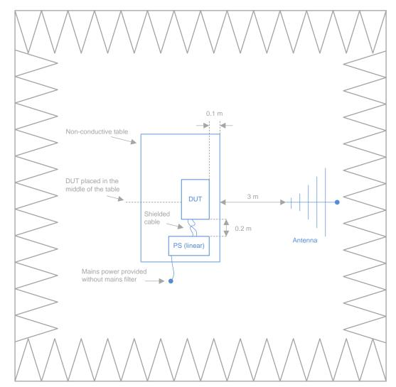
Figure 5. Test Arrangement for Tabletop Equipment According to CISPR 22
