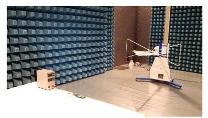
Figure 6. Test Setup: View With Antenna
