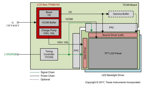
Figure 1. Block Diagram of LCD Subsystem
