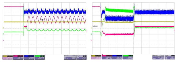
Figure 9. 5-V Output During Crank Test Pulse
