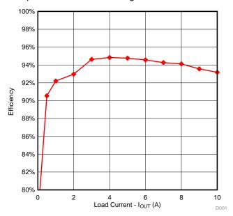
Figure 20. 5-V Output Efficiency
