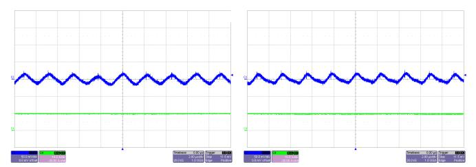
Figure 14. 5-V Output Ripple
