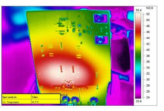
Figure 27. Thermal Measurement at 14-V Input (Back)
