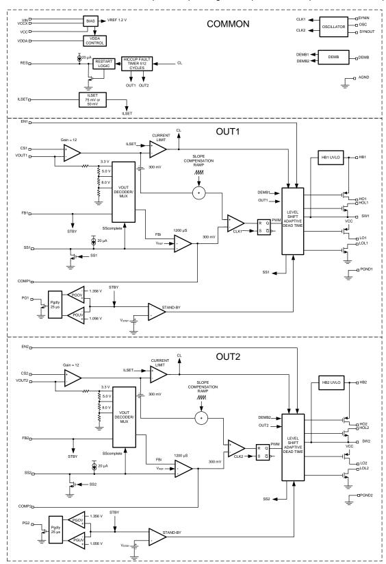
Figure 4. Functional Block Diagram of LM5140-Q1
