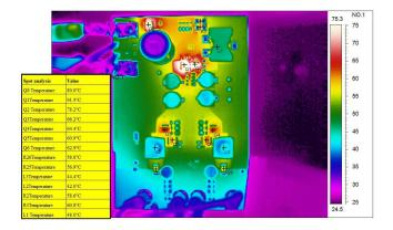
Figure 22. Thermal Measurements at 6-V Input (Front)
