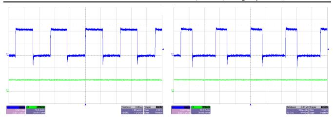
Figure 16. 5-V Output Switch Node
