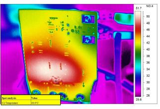
Figure 25. Thermal Measurement at 11-V Input (Back)
