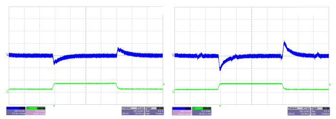
Figure 18. 5-V Output Load Transient Response
