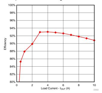
Figure 21. 3.3-V Output Efficiency
