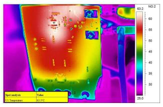
Figure 23. Thermal Measurement at 6-V Input (Back)
