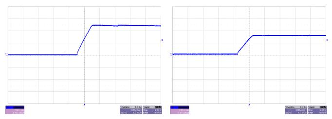
Figure 12. 5-V Output Start-Up (No Load)
