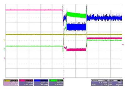
Figure 11. 3.3-V Output During Crank Test Pulse (Zoomed)
