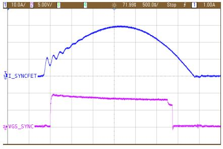
Figure 14. Synchronous Rectifier Working Waveform
