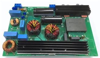
480-W, Thin-Profile (< 17-mm), 94% Efficiency, Fast Transient Response AC/DC SMPS Reference Design
