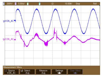
Figure 7. Inrush Current Limiting at Start-Up
