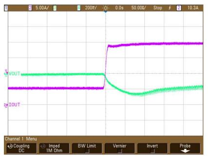
Figure 9. Load Transient Response
