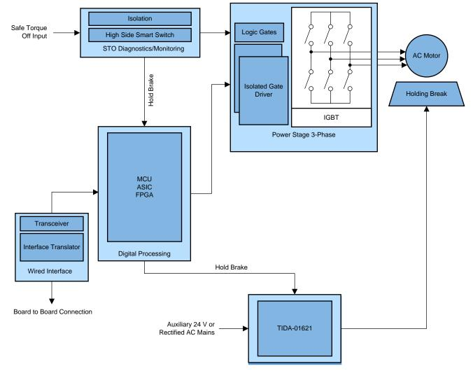
Figure 1. Implementation of Smart-Brake Control in Servo Drives
