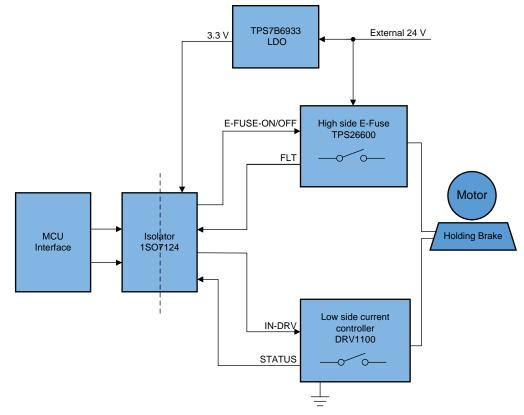
Figure 2. Block Diagram of TIDA-01621
