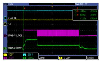
Figure 18. Functionality of E-Fuse, TPS26600
