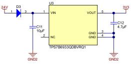
Figure 12. Schematic of TPS7B6933
