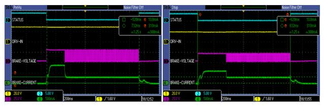
Figure 16. Hold Current of Brake Fixed to 300 mA at 19-V and 28-V Input Voltage
