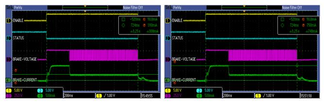
Figure 14. Hold and Peak Currents of Brake Coil
