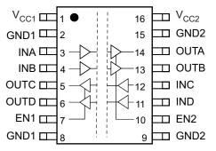
Figure 3. Pin Diagram of ISO7142
