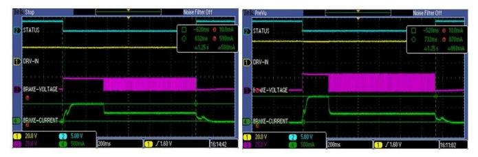
Figure 17. Relative Increase in Peak Current at 19-V and 28-V Input Supply Voltages
