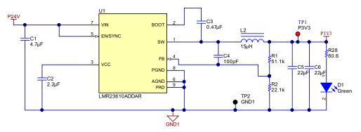
Figure 11. Schematic of LMR23610
