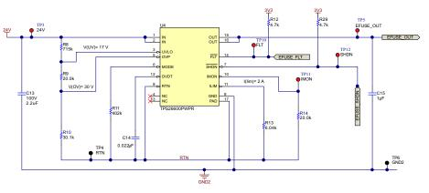
Figure 7. Schematic of High-Side E-fuse
