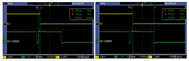
Figure 22. Short-Circuit Event Under Normal Operation of TPS26600
