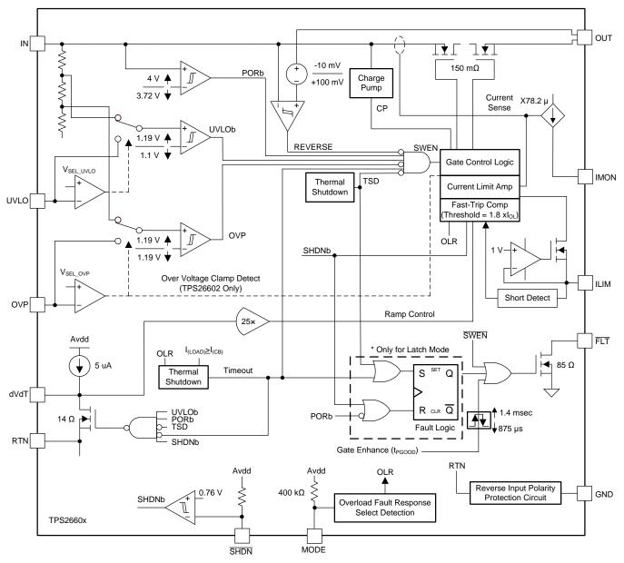
Figure 4. Functional Diagram of TPS26600
