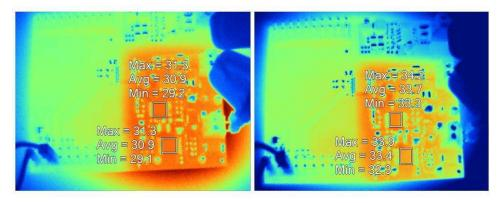
Figure 24. Thermal Image of TIDA-01621 Board
