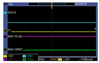
Figure 21. Reverse-Input Polarity Protection at -30 V
