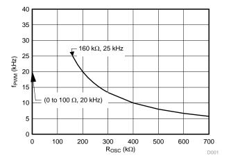
Figure 9. Oscillation Frequency as Function of Resistor Value
