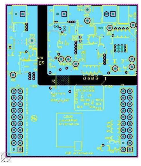
Figure 26. Split in Ground Plane of Layout
