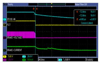
Figure 19. UVLO Threshold for TPS26600
