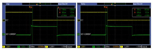
Figure 23. Short-Circuit Event When Circuit Was Originally Open Circuited
