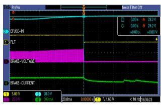
Figure 20. Overvoltage Threshold for TPS26600
