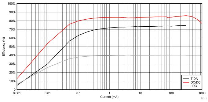
Figure 36. Efficiency Comparison ( $V_{IN} = 3 V$ )
