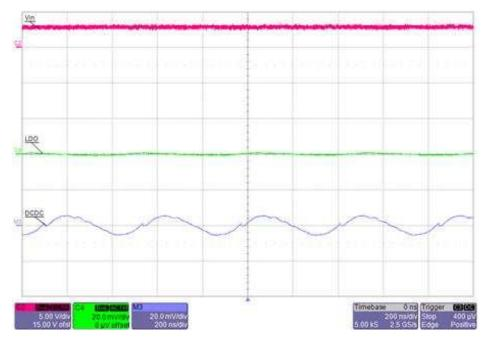
Figure 5. TIDA-01566 Output Ripple (V<sub>in</sub> = 3 V, Load = 100 mA)
