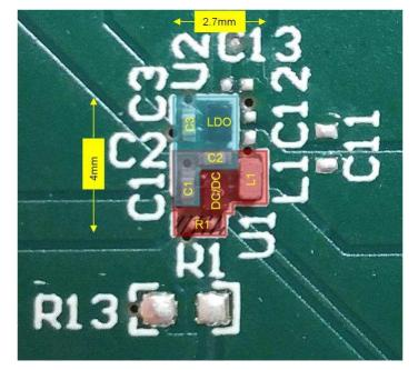
Figure 44. TIDA-01566 Solution Size
