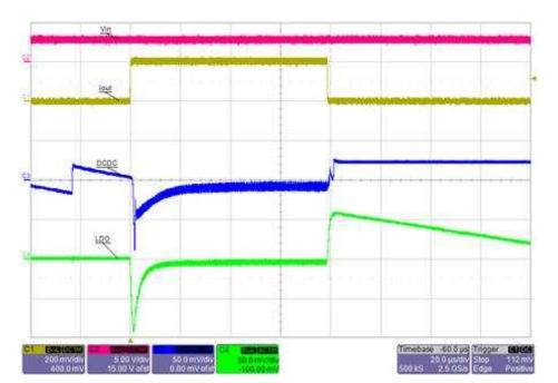
Figure 12. TIDA-01566 Load Transient Response (V<sub>in</sub> = 3 V, 1-mA to 200-mA Load Step)
