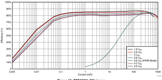
Figure 15. TPS62801 Efficiency
