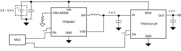
Figure 1. TIDA-01566 Block Diagram
