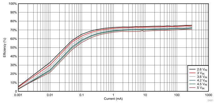
Figure 3. TIDA-01566 Efficiency
