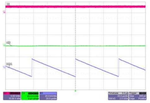
Figure 4. TIDA-01566 Output Ripple (V<sub>in</sub> = 3 V, Load = 1 mA)
