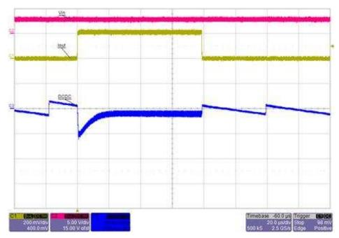
Figure 24. TPS62801 Load Transient Response (V<sub>IN</sub> = 3 V, 1-mA to 200-mA Load Step)
