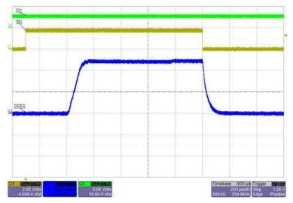
Figure 26. TPS62801 Start-Up and Shutdown ( $V_{IN}$  = 3 V, Load = 0 A)
