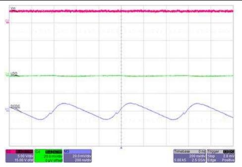
Figure 8. TIDA-01566 Output Ripple ( $V_{in}$  = 3.6 V, Load = 100 mA)
