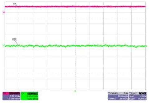
Figure 28. TPS7A10 Output Ripple ( $V_{IN}$  = 3 V, Load = 1 mA)
