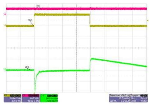
Figure 33. TPS7A10 Load Transient Response (V<sub>IN</sub> = 3 V, 1-mA to 200-mA Load Step)
