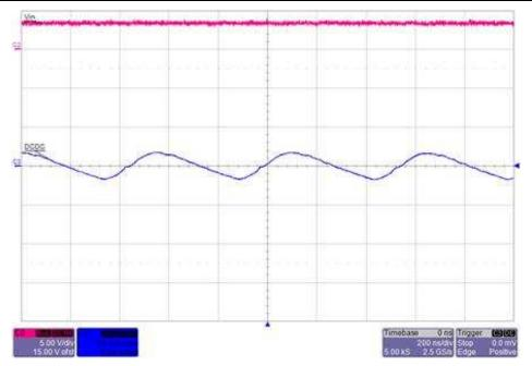
Figure 20. TPS62801 Output Ripple ( $V_{IN}$  = 3.6 V, Load = 100 mA)
