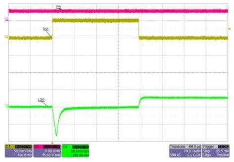
Figure 32. TPS7A10 Load Transient Response (V<sub>IN</sub> = 3 V, 10-µA to 50-mA Load Step)
