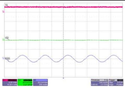
Figure 6. TIDA-01566 Output Ripple (V<sub>in</sub> = 3 V, Load = 300 mA)
