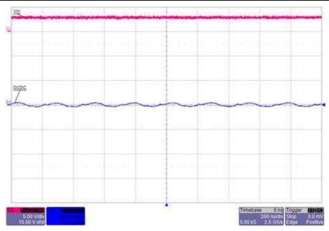
Figure 18. TPS62801 Output Ripple ( $V_{IN}$  = 3 V, Load = 300 mA)
