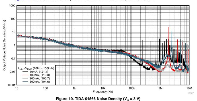
Figure 10 shows the noise density of the TIDA-01566 across multiple load currents.
