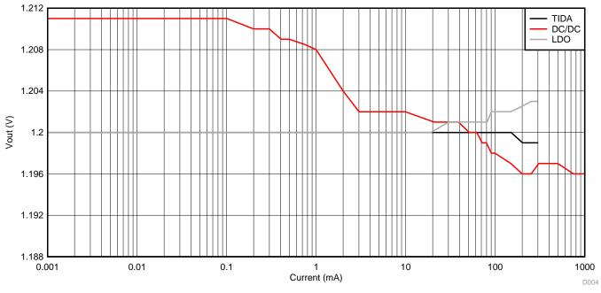
Figure 38. Load Regulation Comparison
