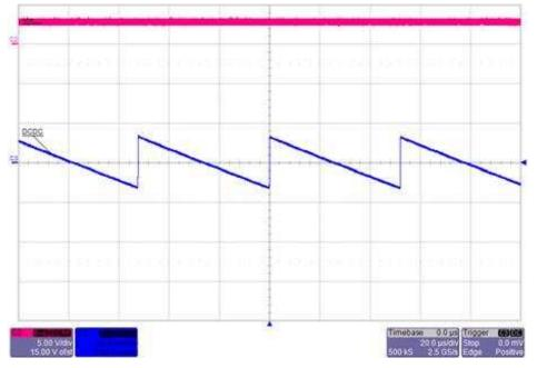
Figure 16. TPS62801 Output Ripple ( $V_{IN}$  = 3 V, Load = 1 mA)
