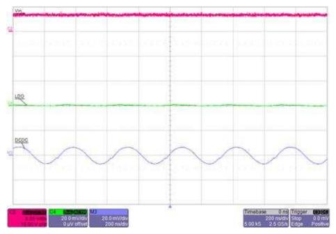
Figure 9. TIDA-01566 Output Ripple ( $V_{in}$  = 3.6 V, Load = 300 mA)
