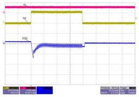
Figure 23. TPS62801 Load Transient Response (V<sub>IN</sub> = 3 V, 10-µA to 50-mA Load Step)
