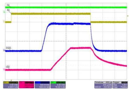
Figure 14. TIDA-01566 Start-Up and Shutdown ( $V_{IN}$  = 3 V, Load = 0 A)
