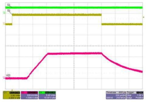
Figure 35. TPS7A10 Start-Up and Shutdown ( $V_{IN}$  = 3 V, Load = 0 A)
