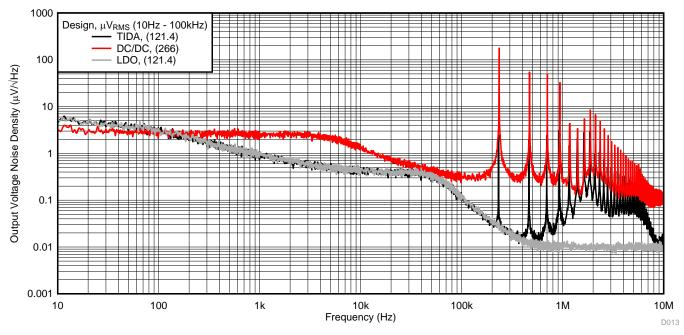
Figure 40. Noise Density Comparison (V<sub>in</sub> = 3 V, Load = 10 mA)
