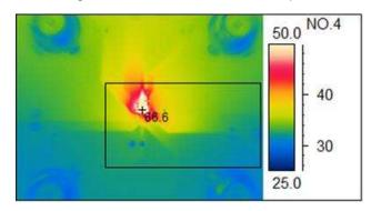
Figure 34. TPS7A10 Thermal Performance ( $V_{IN}$  = 3 V, Load = 300 mA)
