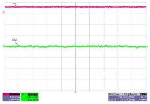
Figure 29. TPS7A10 Output Ripple ( $V_{IN}$  = 3 V, Load = 100 mA)
