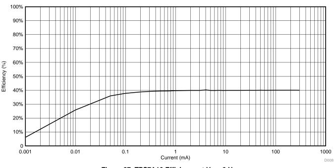
Figure 27 shows the efficiency of the TPS7A10 with a 3-V input. The load is swept from 1  $\mu$ A to 300 mA.
