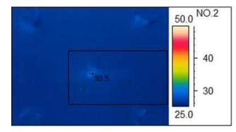
Figure 25. TPS62801 Thermal Performance ( $V_{IN}$  = 3 V, Load = 300 mA)
