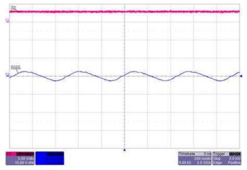
Figure 17. TPS62801 Output Ripple ( $V_{IN}$  = 3 V, Load = 100 mA)
