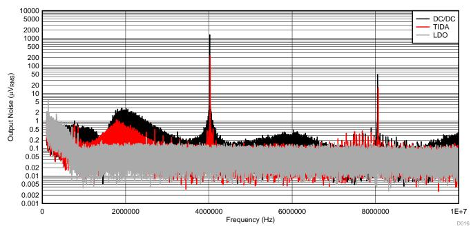
Figure 43. Spurious Noise Comparison (V<sub>in</sub> = 3 V, Load = 300 mA)
