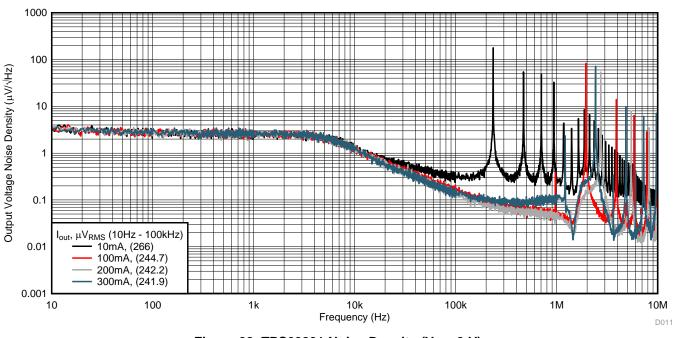
Figure 31 shows the noise density of the TPS62801 across multiple load currents.
