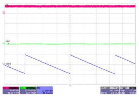
Figure 7. TIDA-01566 Output Ripple ( $V_{in}$  = 3.6 V, Load = 1 mA)
