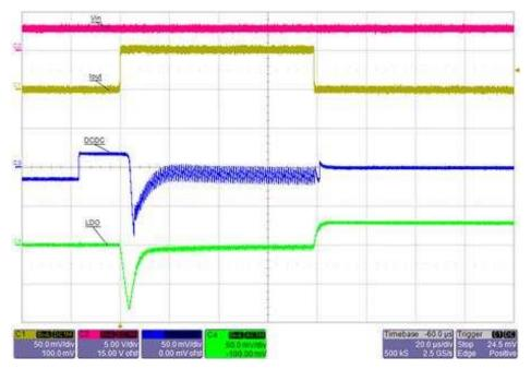
Figure 11. TIDA-01566 Load Transient Response (V<sub>in</sub> = 3 V, 10-µA to 50-mA Load Step)
