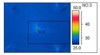
Figure 13. TIDA-01566 Thermal Performance ( $V_{IN}$  = 3 V, Load = 300 mA)
