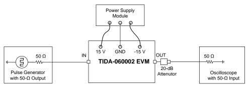
Figure 19. Pulse Response Setup
