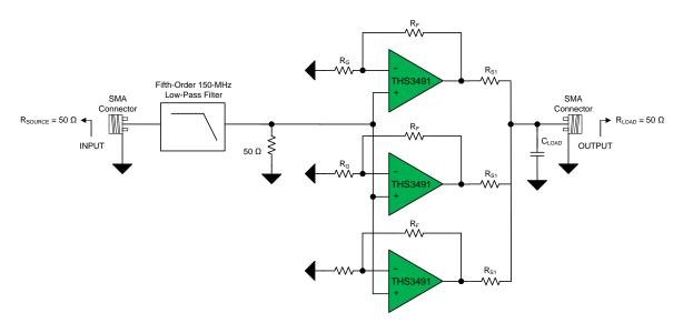
Figure 23. Three THS3491 Parallel Amplifiers Driving a Capacitive Load (CLOAD)
