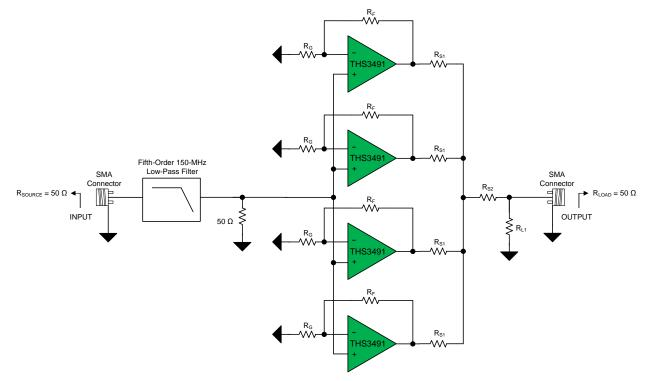
Figure 24. Four THS3491 Parallel Amplifiers Driving a Resistive Load (R<sub>LOAD</sub>)
