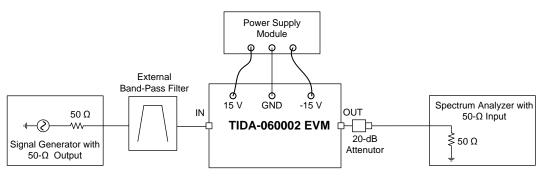
Figure 18. Harmonic Distortion Setup
