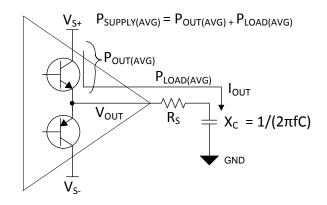
Figure 11. Output Structure for an RC Load (Source Phase)
