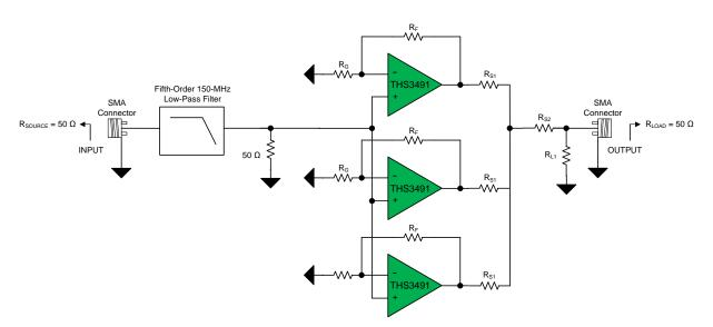
Figure 22. Three THS3491 Parallel Amplifiers Driving a Resistive Load (R<sub>LOAD</sub>)
