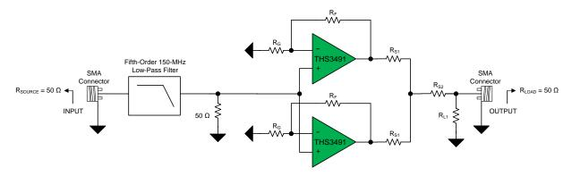
Figure 20. Two THS3491 Parallel Amplifiers Driving a Resistive Load (R<sub>LOAD</sub>)
