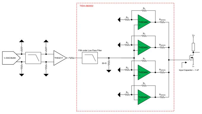
Figure 1. TIDA-060002 Block Diagram
