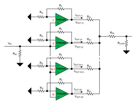
Figure 2. N THS3491 Amplifiers in a Load-Sharing Configuration
