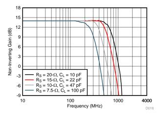
Figure 3. Flat Frequency Response Using Different R<sub>s</sub> for a Given C<sub>L</sub> (Single THS3491)
