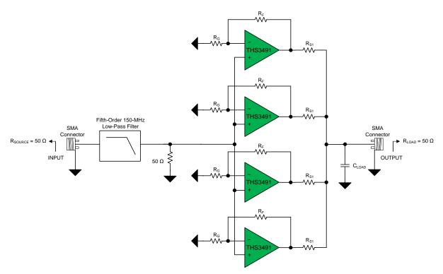
Figure 25. Four THS3491 Parallel Amplifiers Driving a Capacitive Load (C<sub>LOAD</sub>)
