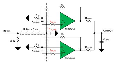
Figure 4. Input Series Resistor (R<sub>DE q</sub>) for Eliminating High-Frequency Oscillation
