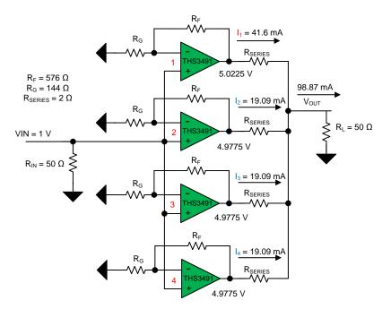
Figure 7. Example Output Current Mismatch Resulting From Output Offset Voltage
