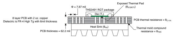
Figure 12. TIDA-060002 PCB Cross Section of Different Thermal Resistances
