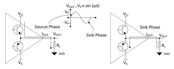
Figure 8. THS3491 Class AB Output Structure
