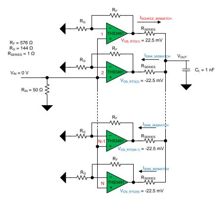
Figure 6. Output Current Mismatch for *N* Load-Sharing Amplifiers
