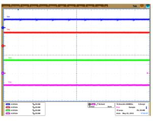
CH1: input voltage CH2: regulated voltage CH3: positive output voltage CH4: negative output voltage
