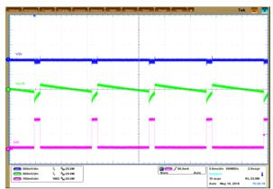
CH1 12-V input voltage CH2: LP8556 backlight output voltage CH3: LP8556 backlight switching waveform CH4: LP8556 output current
