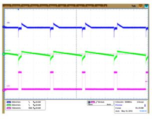
CH1 TPS61089 output 5 V CH4: LP8556 output current CH3: LP8556 backlight output voltage
