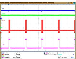
CH1 TPS61089 output 5 V CH2: LP8556 backlight output voltage CH3: LP8556 backlight switching waveform LP8556 output current
