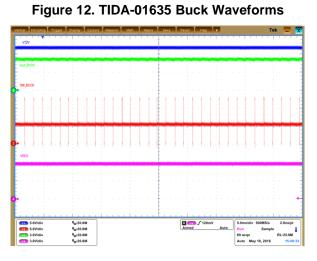
CH1 12-V input voltage CH2: TPS563201 5-V output
