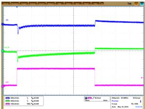
CH1: TPS61089 output 5 V CH4: LP8556 output current CH3: LP8556 backlight output voltage
