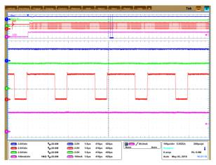
CH1: input voltage CH2: TPS61089 output 5 V CH3: TPS61089 switching waveform CH4: LP8556 output current
