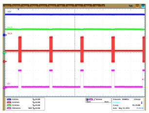
CH1 12-V input voltage CH2: LP8556 backlight output voltage CH3: LP8556 backlight switching waveform CH4: LP8556 output current
