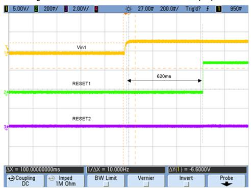
Figure 13. Fault Current Detection for 50-mA DC Step Input
