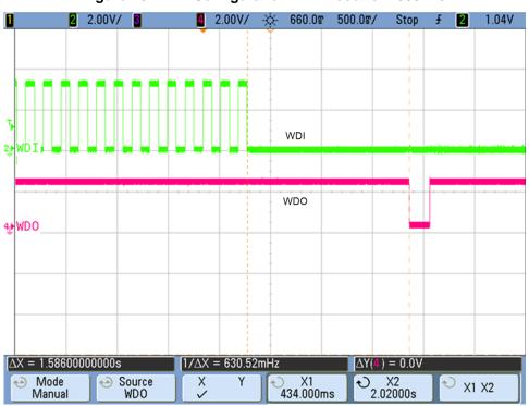
Figure 26. WDT Configuration 2: Timeout of 1600 ms
