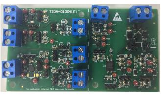
Nano Power, Wide V<sub>IN</sub> (12 V max) Supervisor Reference Design Used as Comparator or Power Sequencer Copyright © 2018, Texas Instruments Incorporated
