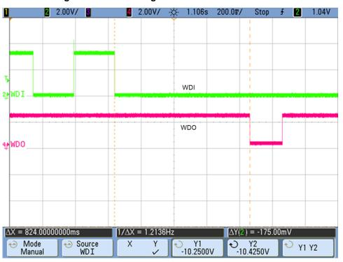
Figure 27. WDT Configuration 3: Timeout of 830 ms
