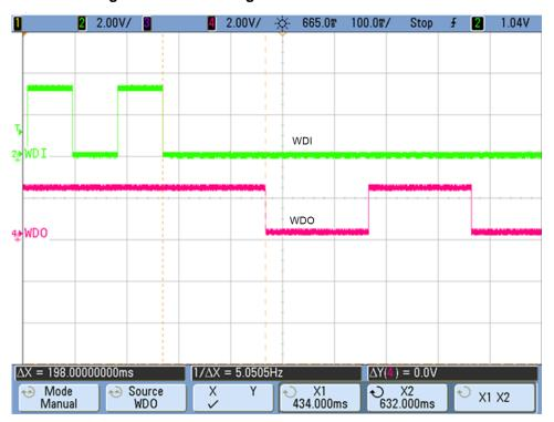
Figure 25. WDT Configuration 1: Timeout of 200 ms
