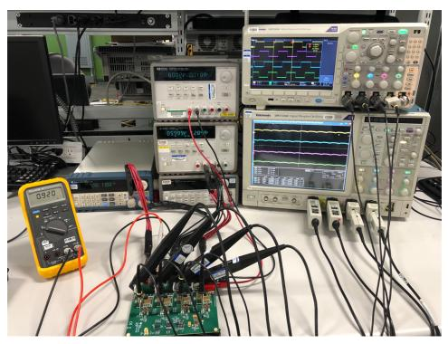
Figure 19. Test Setup and Operation at 6-A Load
