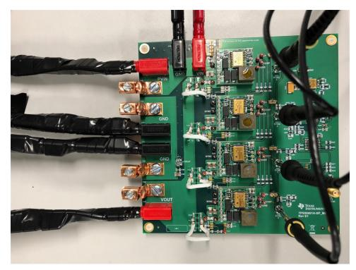
Figure 17. PVin and Vin Power Connections (Power Option 2)
