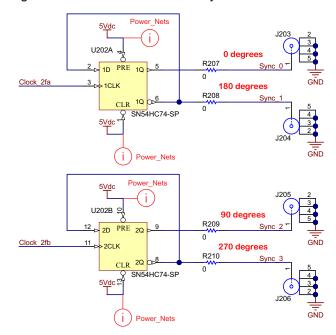
Figure 5. SN54HC74-SP Design Schematic
