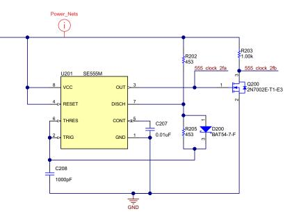
Figure 3. SE555-SP Design Schematic
