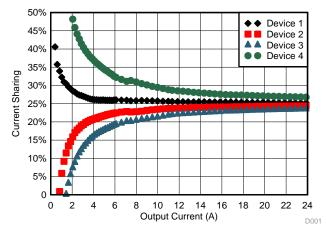
Figure 20. Current Sharing Results Out to 24 A in Quadrature Operation
