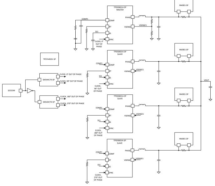
Figure 1. TIDA-070005 Block Diagram
