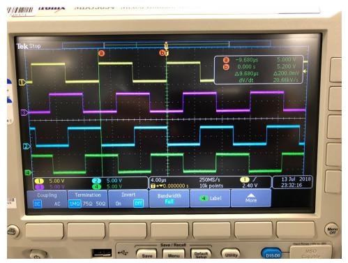
Figure 16. Quadrature Clock Verification
