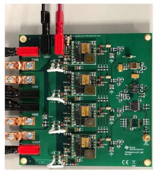
Figure 18. Vin\_LDO\_6V Power Connections (Power Option 2)
