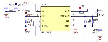
Figure 7. INA901-SP Design Schematic
