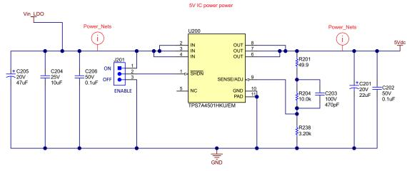
Figure 2. TPS7A4501-SP Design Schematic
