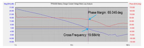
Figure 15. Voltage Close Loop Stability
