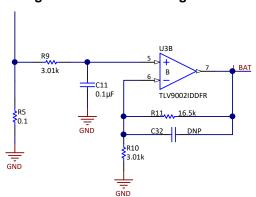
Figure 7. Current-Sensing Circuit
