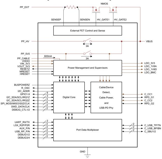
Figure 5. TVS3300 Functional Block Diagram
