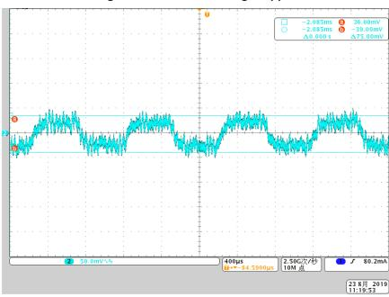
Figure 11. CV Mode Voltage Ripple
