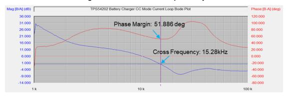
Figure 16. Current Close Loop Stability
