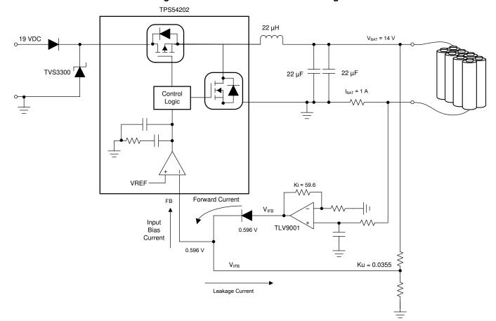
**Figure 6. Constant Current Control Design**
