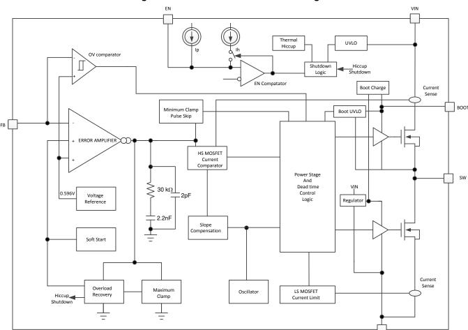
Figure 4. TPS54202 Functional Block Diagram
