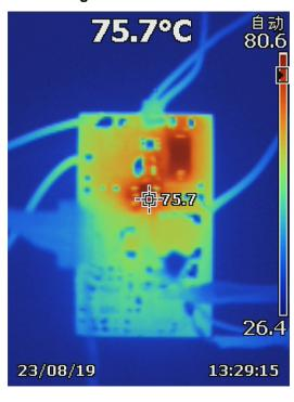
Figure 14. Thermal Test
