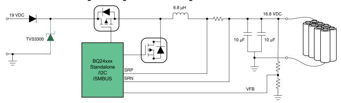
Figure 2. Integrated Onboard Charger Based on BQ24xxx
