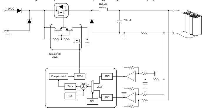
Figure 1. Asynchronous Buck Topology Charger Controlled by System MCU
