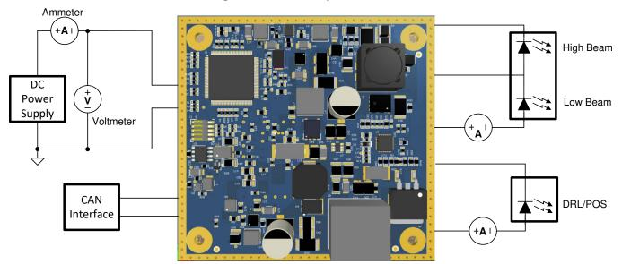
**Figure 10. Test Setup Connections**
