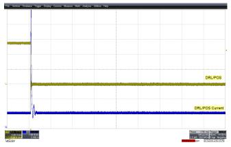
Figure 24. DRL/POS Open Protection
