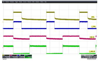
Figure 19. 90% PWM'ing at Low Power
