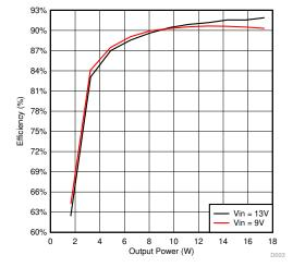
Figure 29. DRL (ILED = 1 A) Efficiency vs P<sub>OUT</sub> (W) 90% 87.5% 85% 82.5% 80% Efficiency (%) 77.5% 75% 72.5% 70% 67.5% Vin = 13V Vin = 9V 65% 2 4 6 16 18 20 10 12 14 8 Output Power (W)
