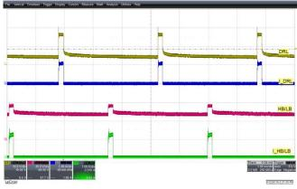
Figure 20. 50% PWM'ing at Low Power
