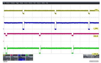
Figure 18. 10% PWM'ing at High Power
