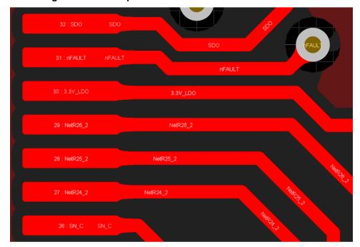
Figure 26. Teardrops Used on Transitions From Vias to Pads
